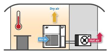
Room temperature is at or above set point. Dehumidifier dries the room without heating. Heat is expelled outside.
