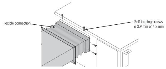
Air duct fixing at the supply and return ports
